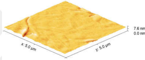
Figure 4.27. 3D AFM image of the sample that contains 20 ML AlSb IMF layer and post annealed at 550 °C. The RMS value is determined as 0.4 nm.
