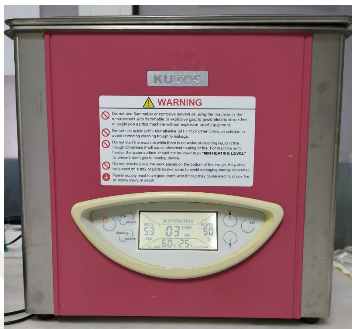
Figure 2. 1 The used ultrasonic bath for substrate cleaning
