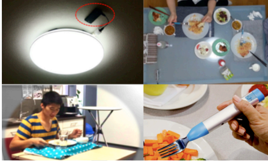
Figure 2.2: Top row images show the ceiling light camera and a typical taken photo. The bottom-left image is showing the smart table surface. The HAPIfork is shown in the bottom-right picture.
