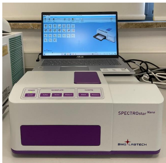
Figure 3.2. Image of UV-vis spectrophotometer device used in the analysis.
