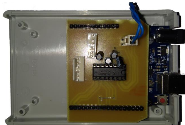
Figure 5.4 RS232 converter module (Personal archive, 2018)
