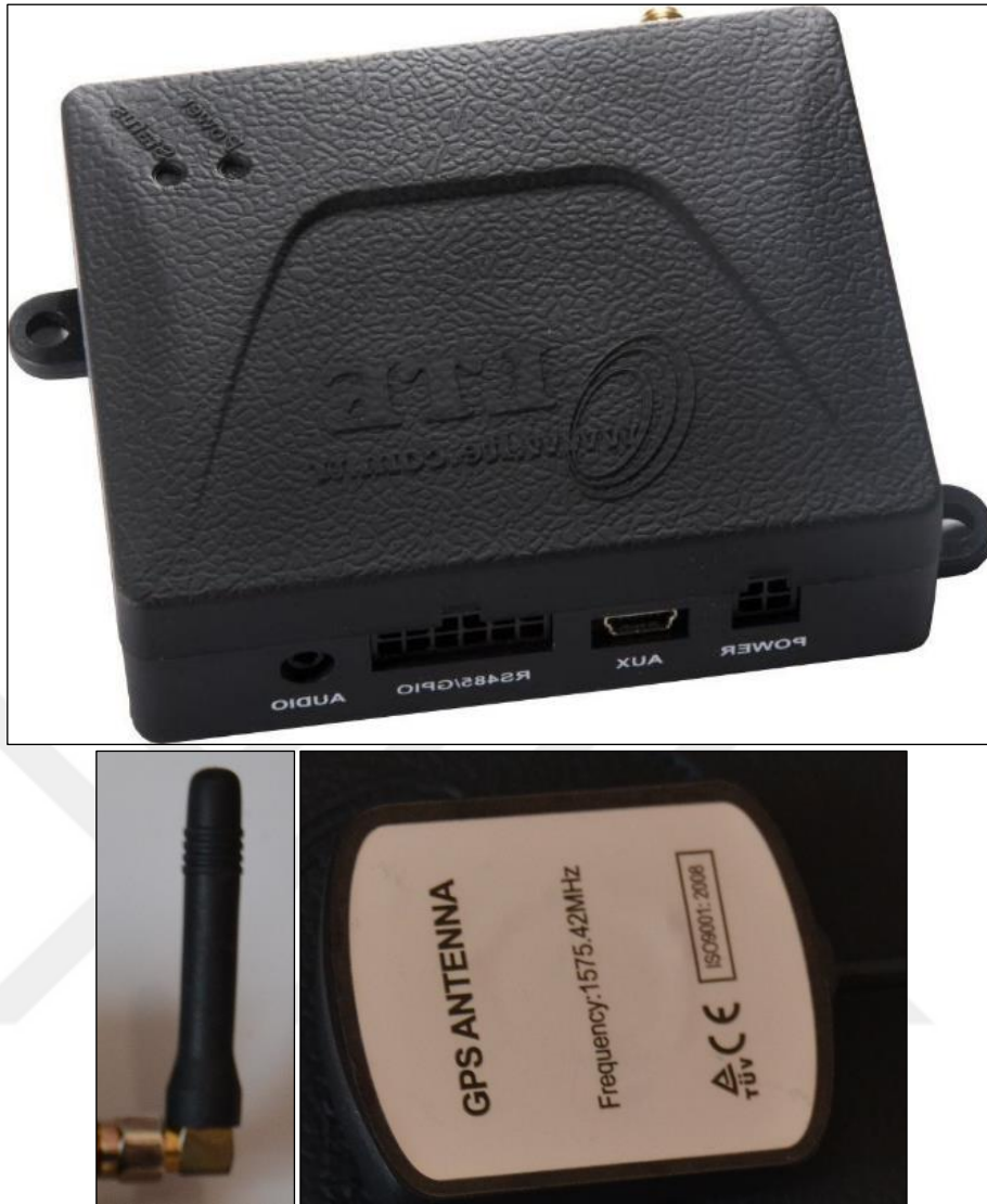
Figure 5.1 HE910T-3G GSM/GPS module (Personal archive, 2018)
