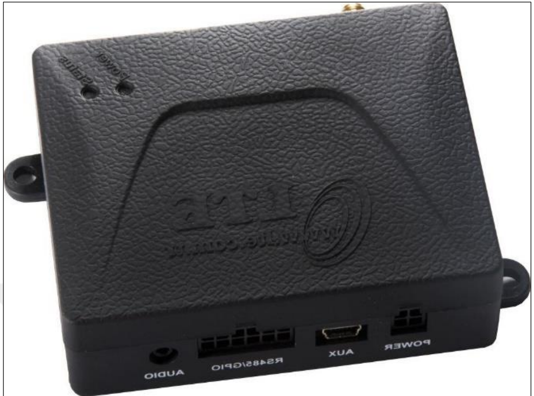
Figure 2.6 HE910T-G GSM/GPS module (Personal archive, 2018)
