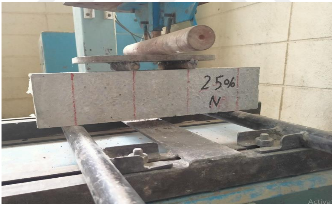
Figure 3.17: Flexural Test Samples.
