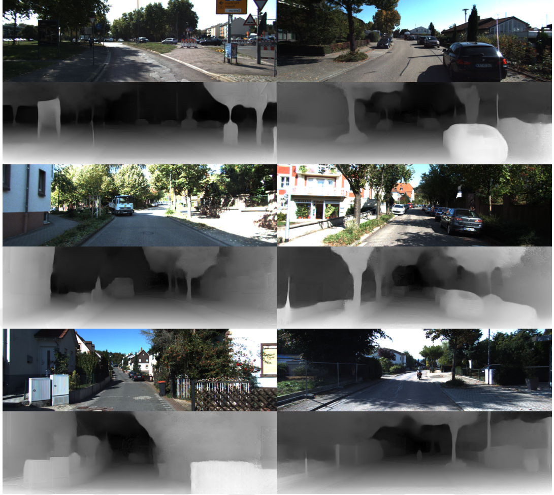
Figure 4.10: Some images and their depth estimation when Monodepth2 is trained BA mimicking method described in Section 4.3.4
