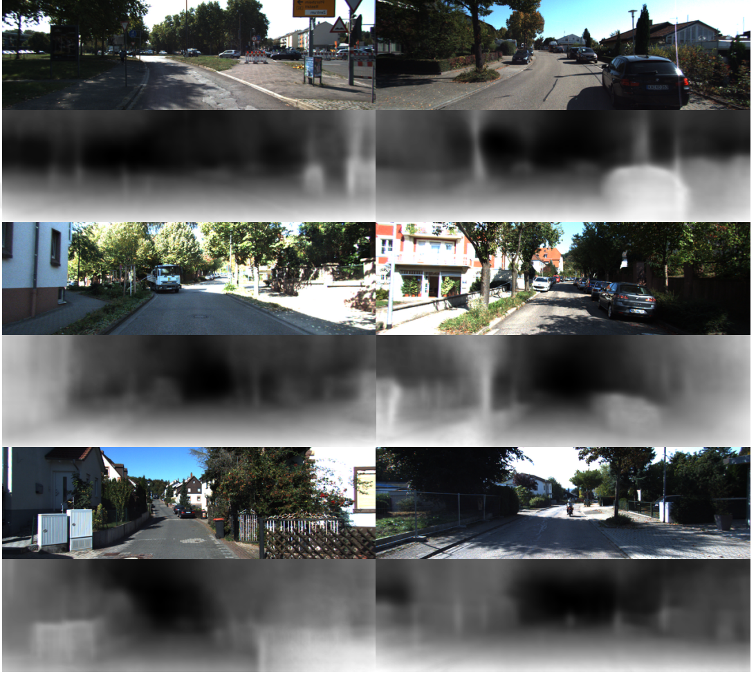
Figure 4.4: Disparity estimation results for Monodepth2 whose network is trained by using COLMAP pose estimates. (Bright regions indicate closer points)
