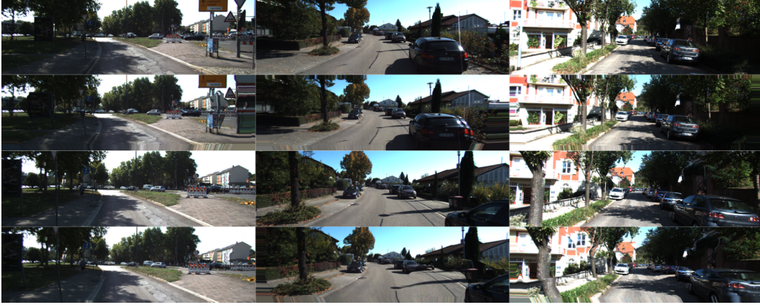
Figure 4.9: The first row shows the images I_0 , the second row show I_0 's prediction from I_{+1} , the third row shows the I_{+5} and the fourth row shows the prediction of I_0 from I_{+5}
