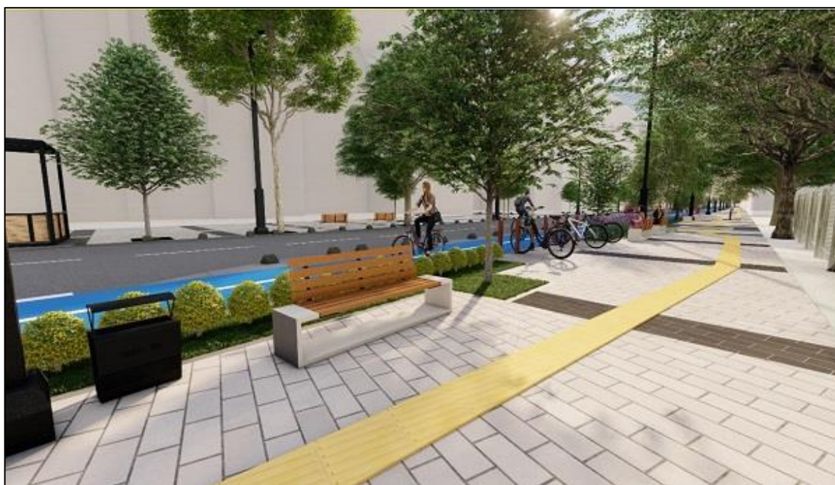
Figure 5.31. Bench and garbage can design placed on the sidewalks. [107]
