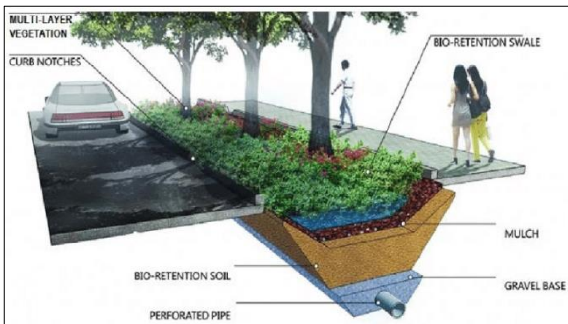
Figure 5. 52. Example of a rain ditch [15].
