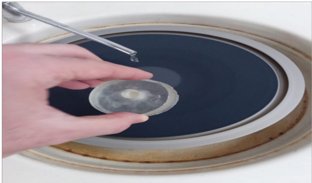
Figure 2.7. Preparing the specimen for the other mechanical tests by polishing it to create a smooth surface
