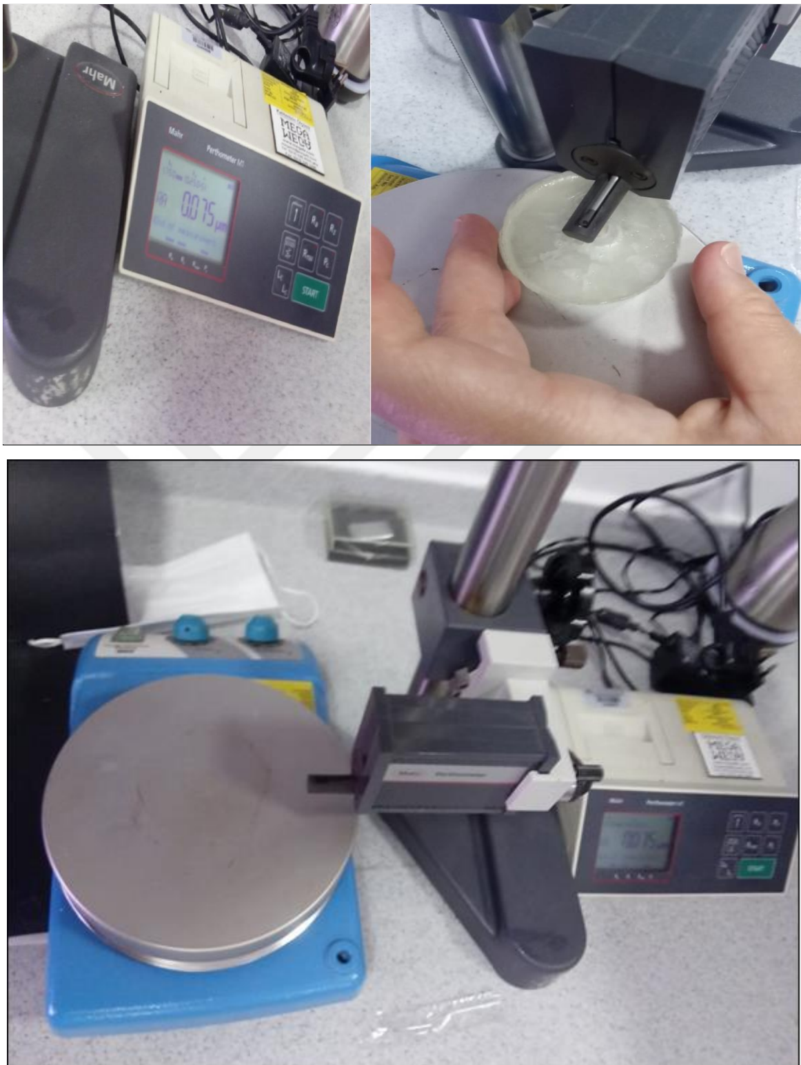
Figure 2.9. A measurement screen and a Perthometer M1 surface roughness tester from Mahr in the Czech Republic
