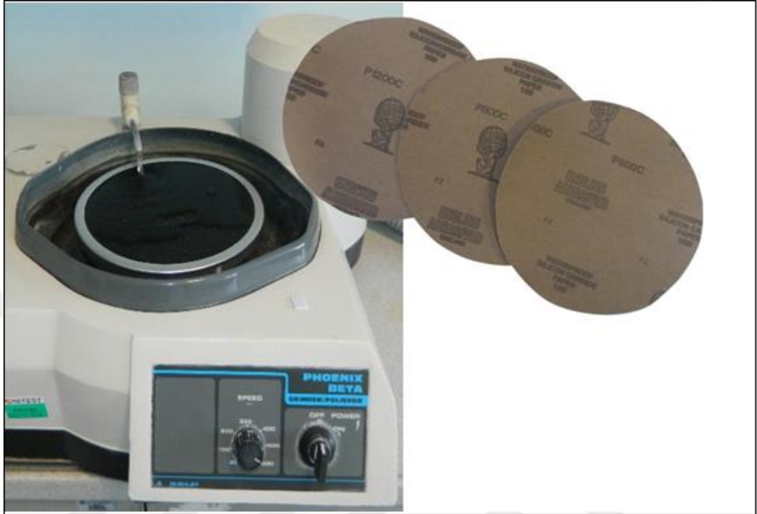
Figure 2.6. Silicone carbide sandpapers and polishing machines with granulometry of up to 2500, 1200, and 600 meshes, respectively
