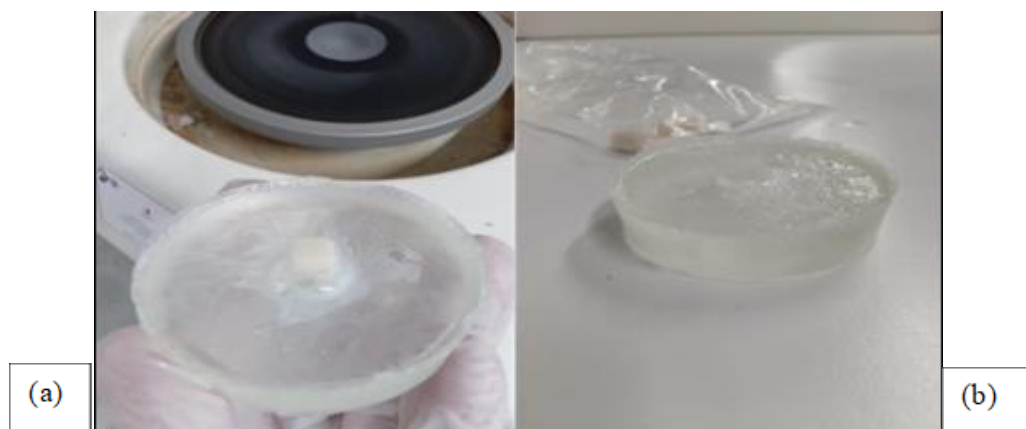
Figure 2.5. Sample mould which was mad from a combination of Epocold –R (Epoxy cold mounting resin) and Epocold – H (Epoxy cold mounting resin).
