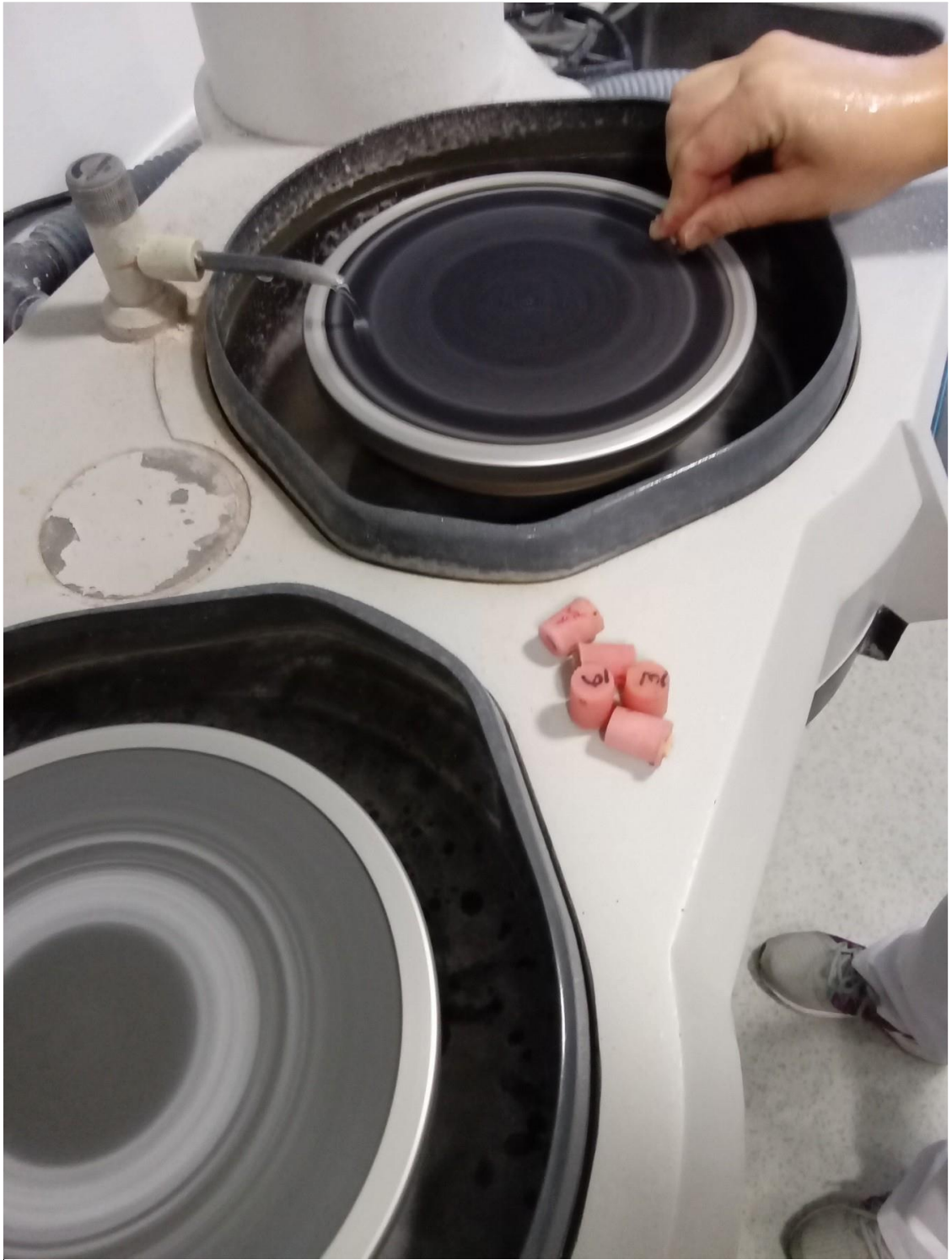
Figure 2.2. Pink part removal using sand paper machine
