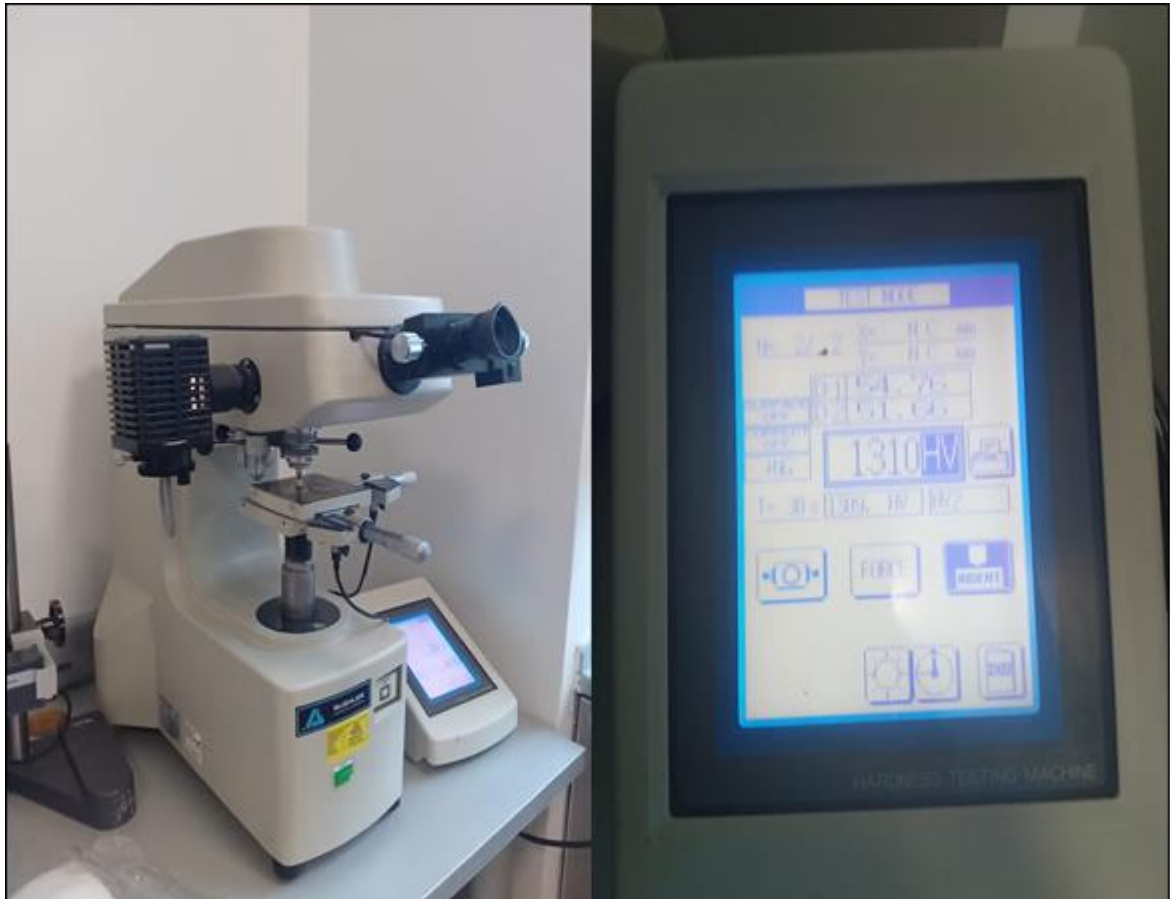
Figure 2.10. Vickers hardness device (Buehler Britain Ltd., England), and a screenshot of the result interface
