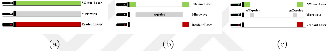
Figure 4.3: Comparison of sensing modalities: (a) CW-ODMR, (b) Single MW Pulsed-ODMR, and (c) Ramsey Pulsed-ODMR. Adapted from the schematic in Ref. [4].
