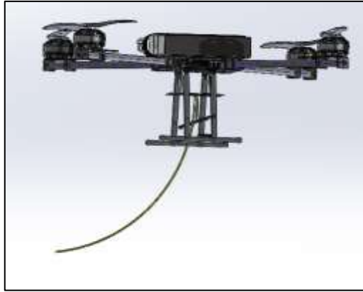
Figure 3.12: Drone Equipped with Tubing for Spraying Operations.
