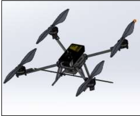
Figure 3.7: The Final Assembly of Quadcopter Drone.
