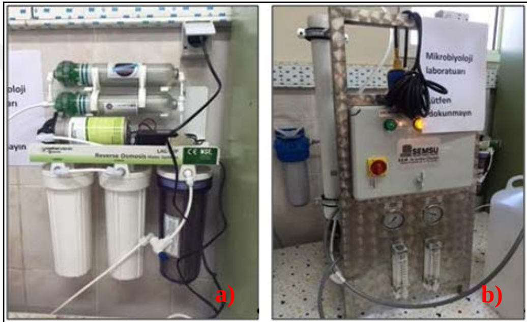
Figure 5.6 Reactor configurations of (a) UF membrane and (b) RO membrane (Personal archive, 2016)
