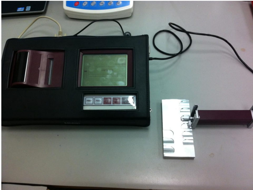
Figure 6.30 – Sample measurement of surface roughness with Mitutoyo SJ-301
