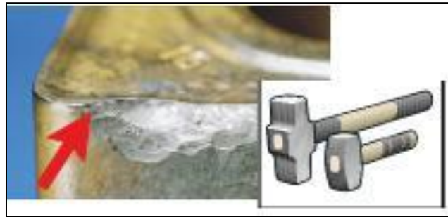
Figure 5.19 – Example chip hammering image
