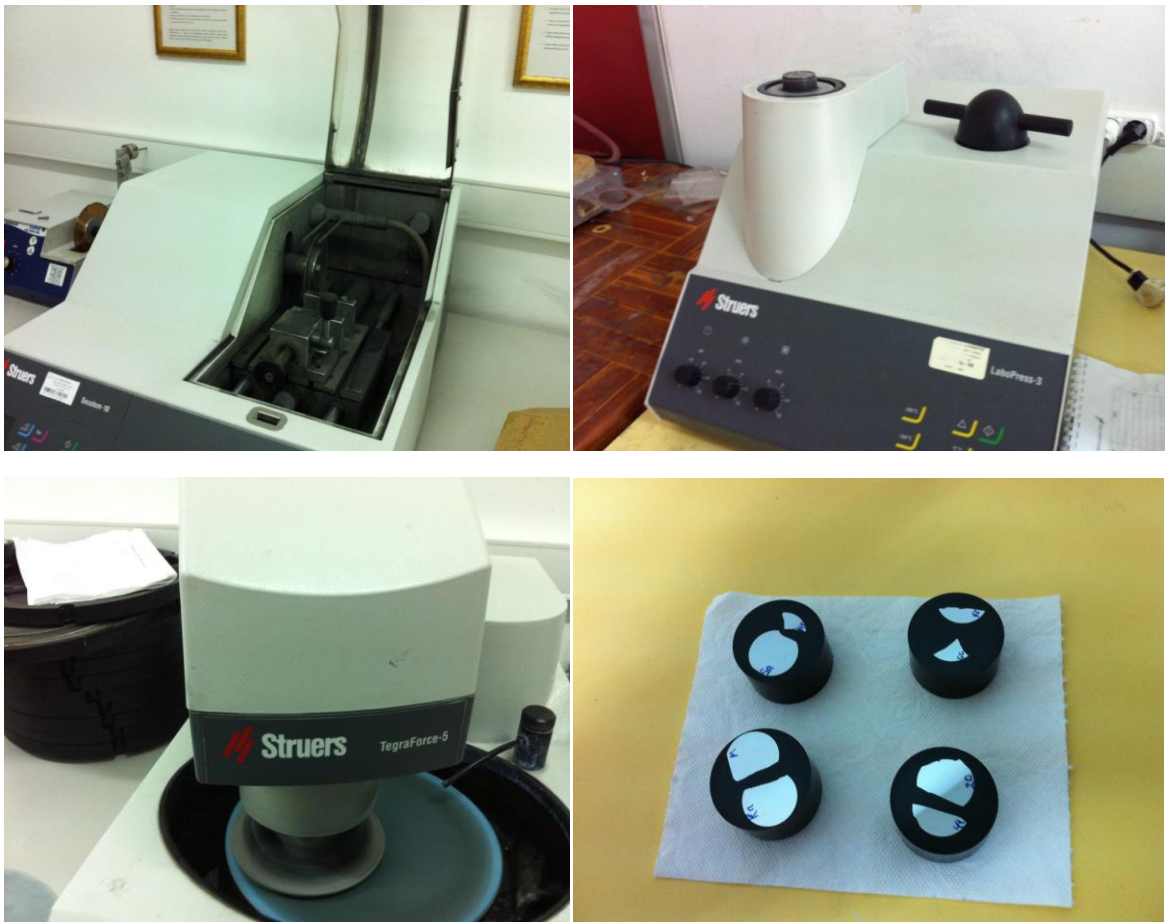
Figure 6.44 – Preparation of the samples for the hardness tests
