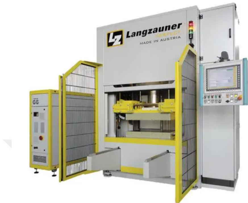
Figure 27. The hydraulic press used in consolidation of CF and PEEK to obtain reinforced composite laminate (source: DirectIndustry & Langzauner).
