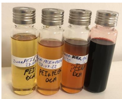
Figure 23. The solvent-based sizing agents prepared by 2wt% polymer dissolved in DCA medium: PEI, PEI-PEEK blend, PEEK, and HPEEK solutions (from left to right).
