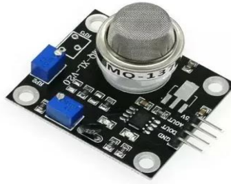
Figure 4: MQ-137 ammonia sensor
