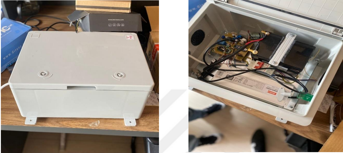
Figure 22: Air quality monitoring system
