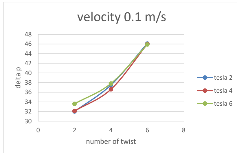
Figure 4.70: Effect Of Cycles Of Rotation And Intensity Of Magnetic Field On Pressure Drop At Velocity 0.1 M/S And Thickness Of Magnetic 70 Mm.
