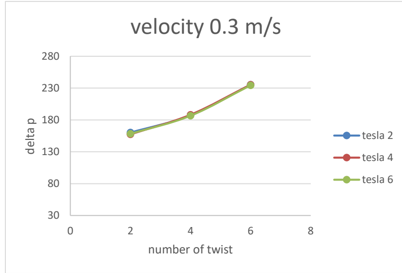
Figure 4.41: Effect Of Cycles Of Rotation And Intensity Of Magnetic Field On Pressure Drop At Velocity 0.3 M/S And Thickness Of Magnetic 50 Mm.
