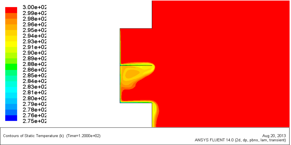
Figure 3.19 Temperature contours of the refrigerator and the opening on it at 1 shelf condition with 2°C starting temperature at 5th and 120th sec.
