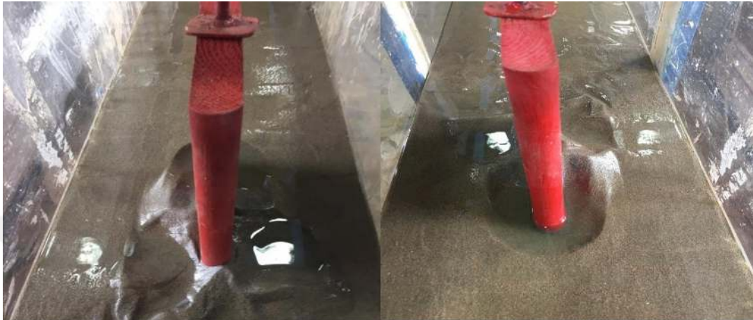
Figure 2.10 Around The Rectangular Pier Rounded Snout is Scour and Dunes.
