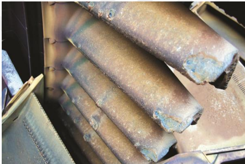
Figure 2.6: Erosion of Gas Turbine Blade [87].
