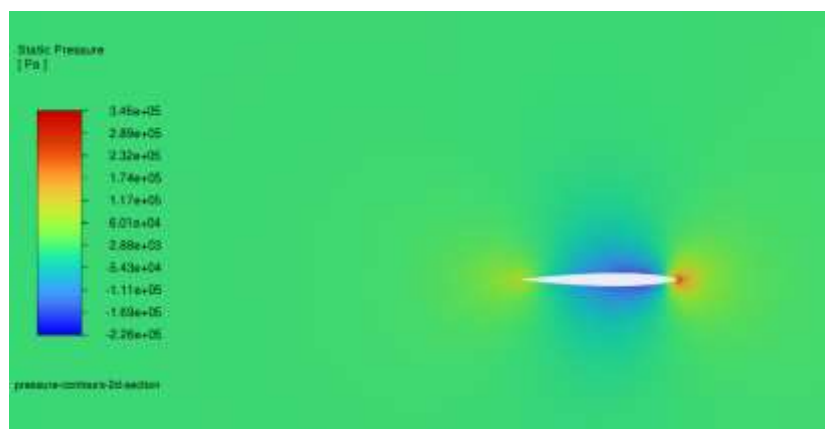
Figure 4.7: Pressure Contours on the 2D Wing Section of the XQ-58A Valkyrie.
