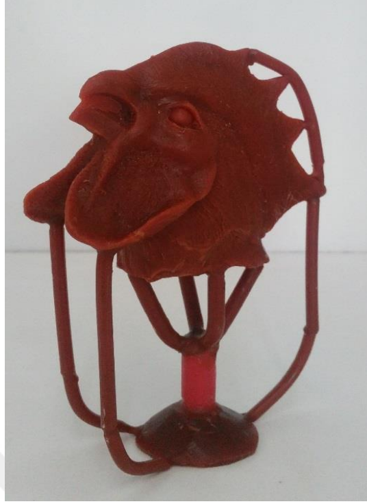
Görsel 2.26. Tepeden Beslemeli Mum Model (Ergün Arslan,2019)
