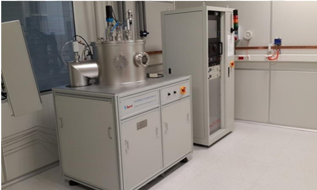
Picture 4. RF magnetron sputtering technique in NÜRDAM at Bolu Abant Izzet Baysal University.
