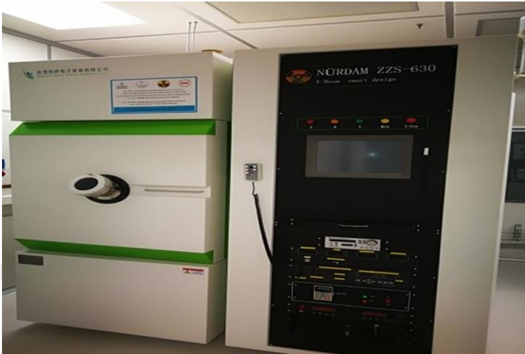
Picture 5. E-beam evaporation technique in NÜRDAM at Bolu Abant Izzet Baysal University.
