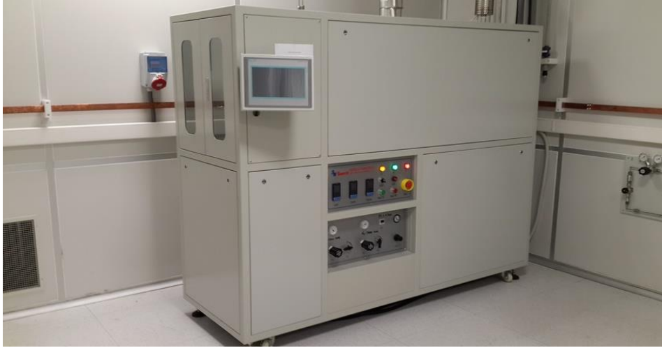
Picture 3. Annealing furnace in NÜRDAM at Bolu Abant Izzet Baysal University.
