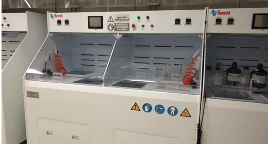
Picture 1. Wet chemical benches for wafer cleaning in NÜRDAM at Bolu Abant Izzet Baysal University.
