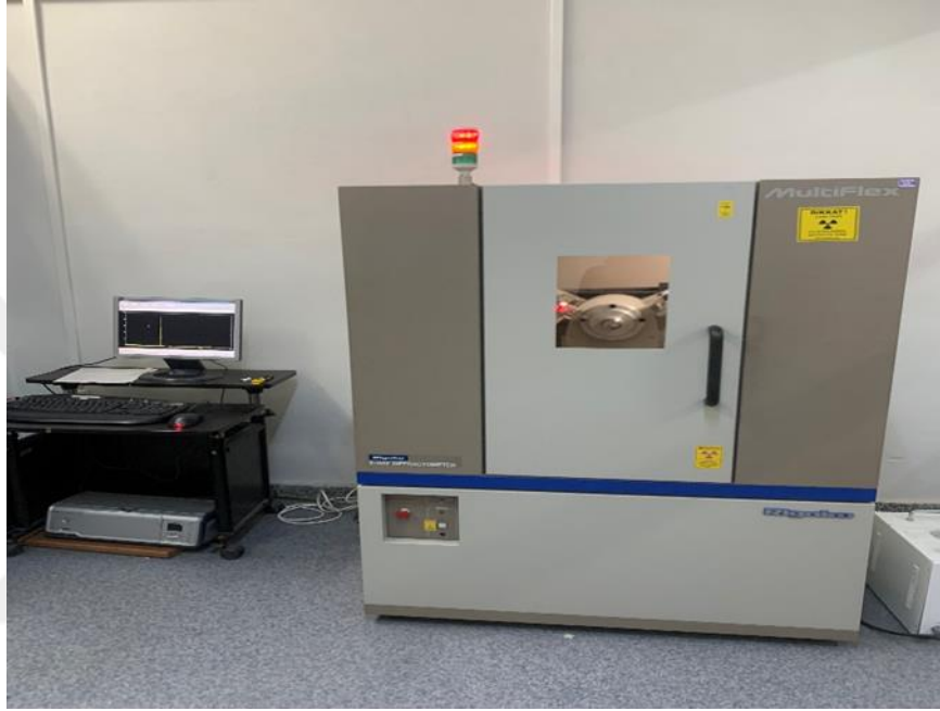
PICTURE 7. Rigaku MultiFlex X-Ray Diffractometer in the Department of Physics at Bolu Abant Izzet Baysal University.
