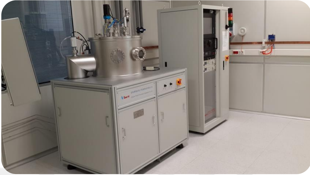
Figure 7.1. The magnetron DC/RF sputtering system in Nuclear Radiation Detector Center (NURDAM) Abant İzzet Baysal University.
