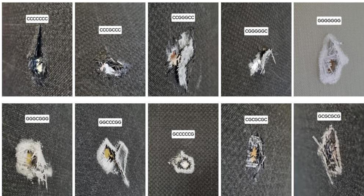
Figure 22. Bullet exit damage on the sample surface
