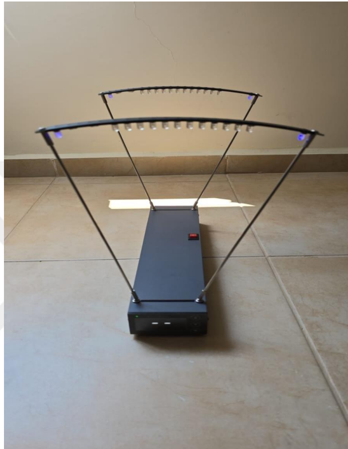
Figure 18. PRECISION BALLISTIC CHRONOGRAPH BULLET SPEED MEASURING DEVICE
