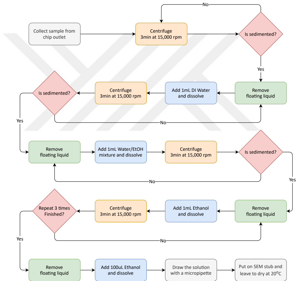
Figure C.1: Washing procedure to remove oil from samples and prepare them for SEM imaging.
