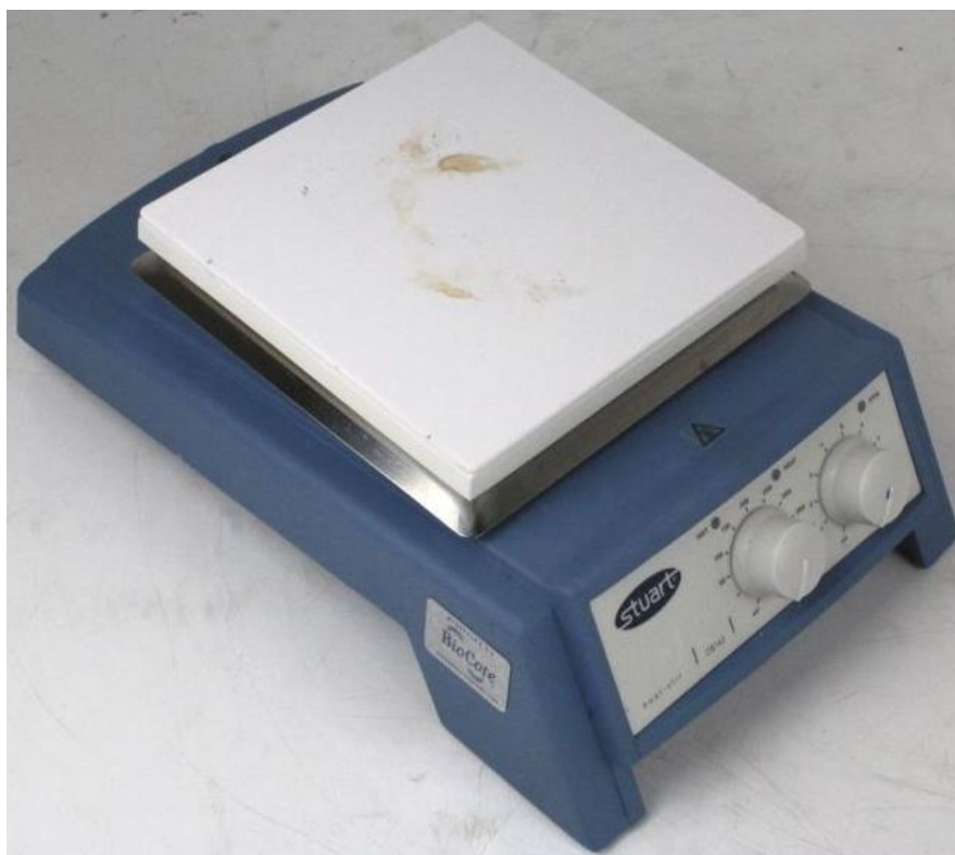
Figure 2.1. Stuart CB162 magnetic stirring hotplate
