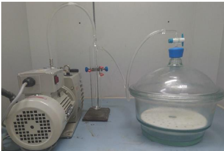
Figure 8: The vacuum set-up used for polymer lyophilization consisting of vacuum pump, connection and desiccator chamber. The desiccator chamber was ensured a tight seal by frequent application of vacuum grease to the chamber and lid lips.
