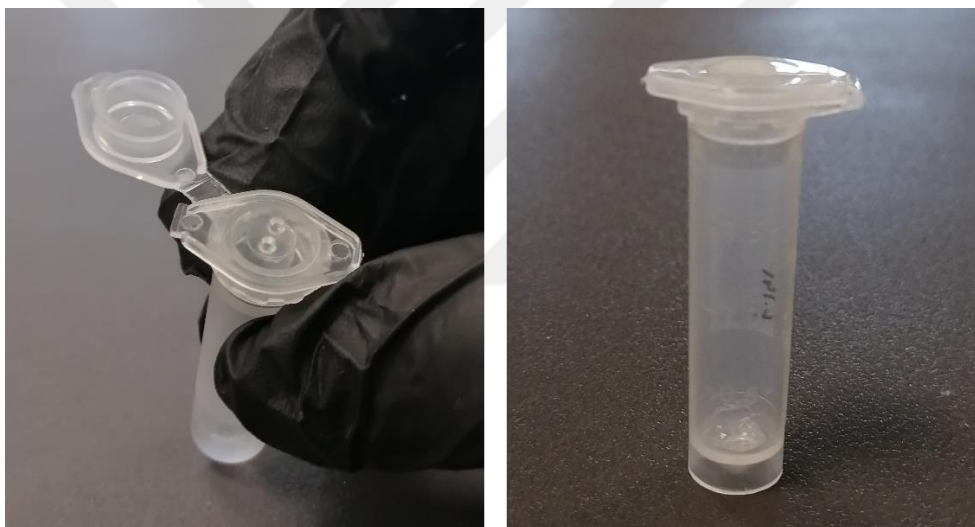
Figure 7: Polymer samples before and after lyophilization. Left: 2 mL Eppendorf tube closed with punctured cap for freezing in liquid nitrogen and subsequent drying under vacuum. Right: sample removed from vacuum and closed with original cap. Lyophilized polymer can be seen as small amount of solid at the bottom of the tube.
