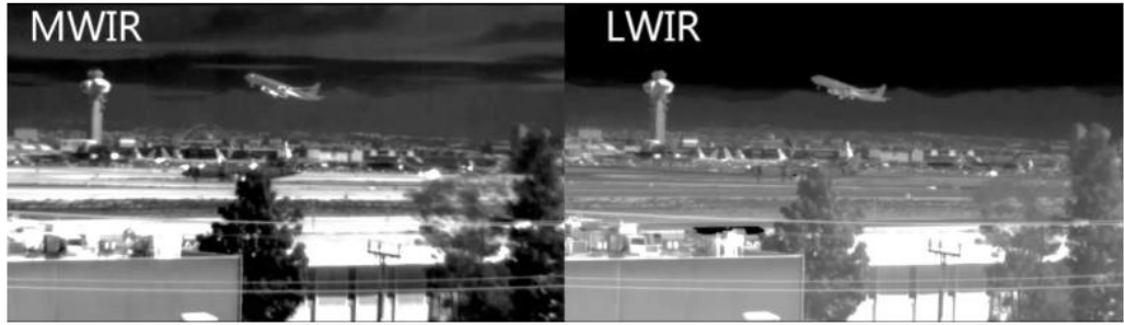
Image 2.5. 1280 \times 720 , 12 \mu\text{m} pixel pitch dual band superlattice FPA images [44].
