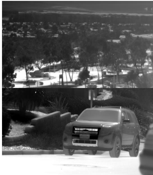
Image 2.6. An image obtained at 150 K with 1\text{k} \times 2\text{k} , 5 \mu\text{m} pixel pitch FPA [45].
