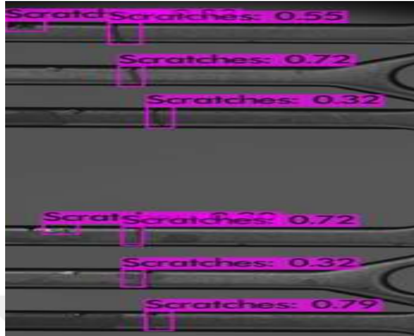
Figure 8.3. Scratches defect prediction output.
