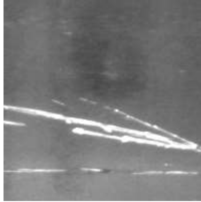
Figure 2.6. Example of scratches defect
