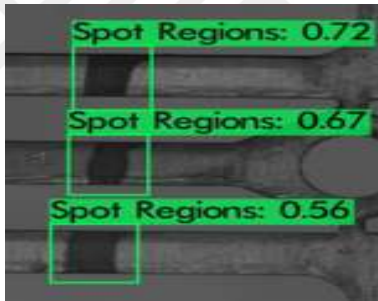
Figure 8.4. Spot regions defect prediction output.
