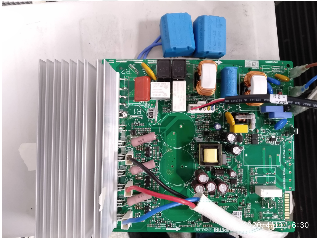
Figure 5.2.1: Inverter board with 10uF film capacitor
