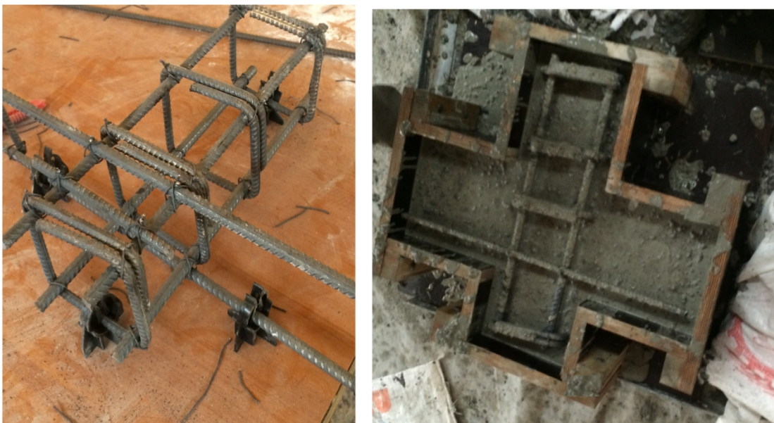
Figure 3.2 Reinforcement of the specimen
