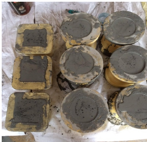
Figure 3.5 Casting of cylinders and cubes
