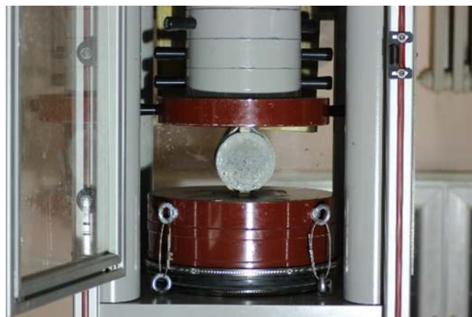
Figure 3.9 Splitting tensile test
