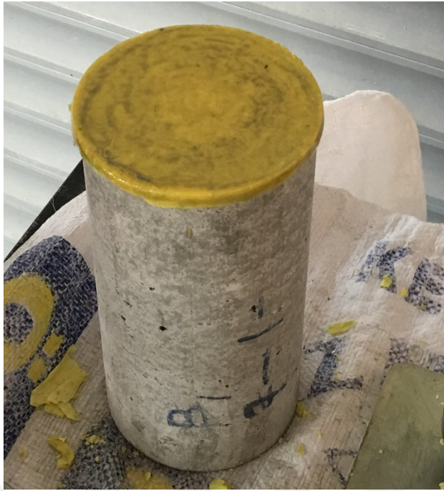
Figure 3.10 Sulfur capped specimen
