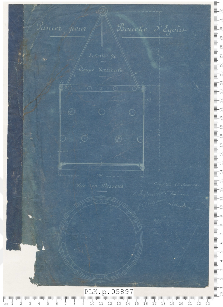
Figure 5.2 Sewer Basket. SOURCE BOA., PLK.p. 5897, 20 March 1913.
