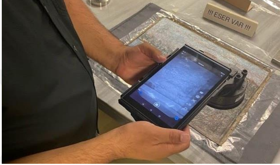
Şekil 3.39: Forenscope marka Mobile Multispectral Forensic Tablet.
