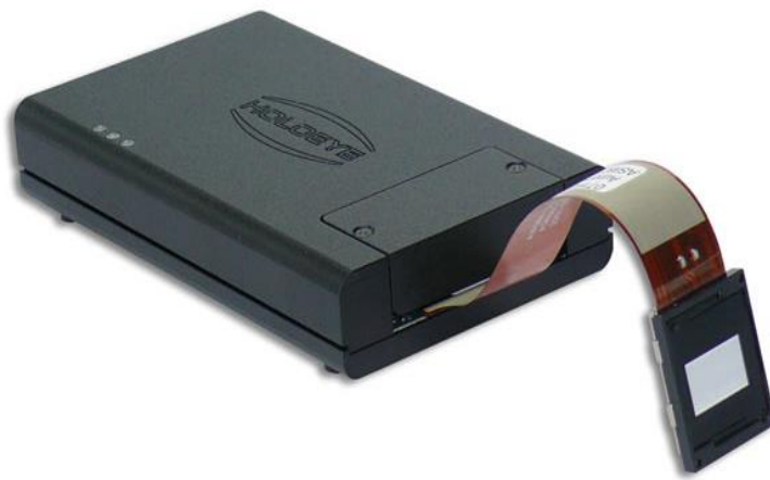
Figure 3.7 : PLUTO-BB SLM manufactured by HOLOEYE.
