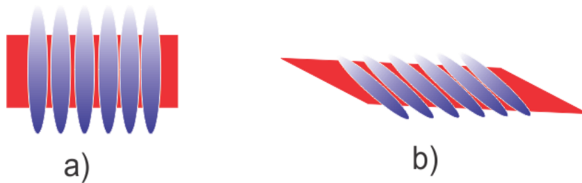
Figure 3.2 : Ferroelectric LC in an external electric field of a) \vec{E} b) -\vec{E}
