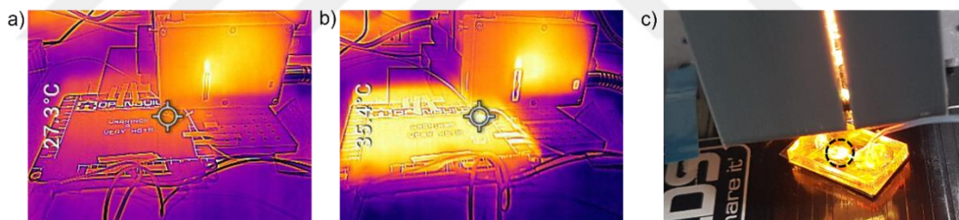
Figure 3.9 Thermal camera images during a) capture at room temperature (~27 °C < LCST of PNIPAM) and b) at higher temperature (~35 °C > LCST of PNIPAM) were validated. c) PNIPAM formation in the channel at 45 °C was also observed.
