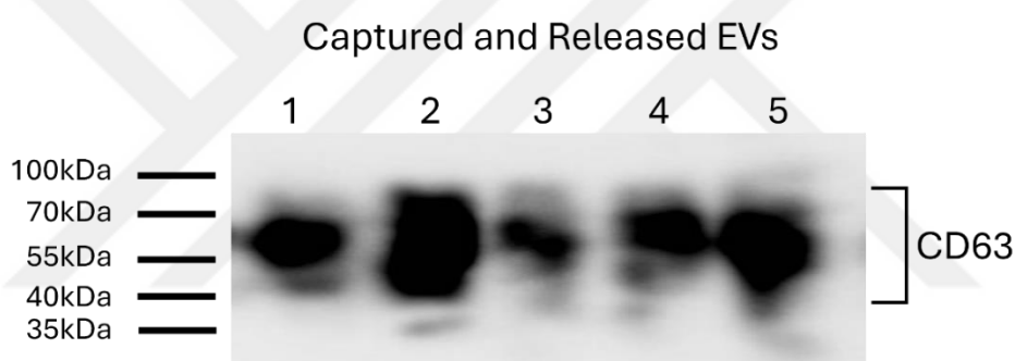
Figure 3.18 Western blot validation of the CD63 tetraspanin protein presence on the EVs released from plasmonic metasurface was depicted.
