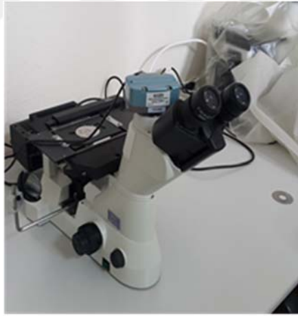
Şekil 0.3 Nikon Eclipse MA100 model ters metal mikroskobu
