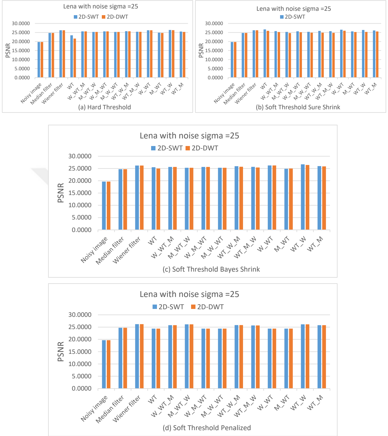
Figure 5.9. PSNR values of the comparison between process steps with (a) Hard, (b) Sure Shrink, (c) Bayes Shrink, and (d) Penalized threshold techniques used, for Lena image, with noise \sigma=25 .
