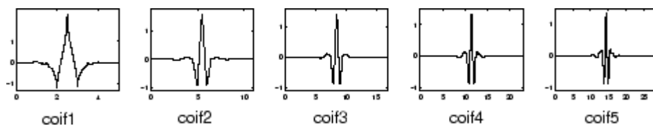
Figure 3.17. The transfer function of the Coiflet wavelet transformation filter family [108].
