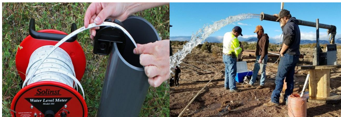
Figure 2.2. Measuring the groundwater level and evaluating the characteristics of the aquifer.
