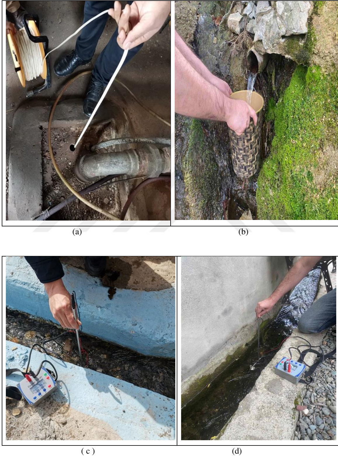
Figure 3.2. Measurement of a) groundwater level in the wells by using a sounder, discharge rates of the springs b) by specific volume method, and c, d) by using of current meter
