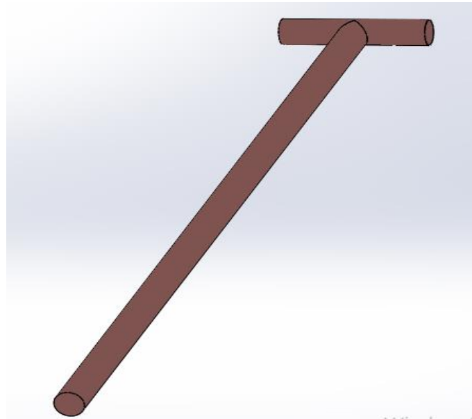
Figure 4.2 Isometric view of the metal inner tube design
