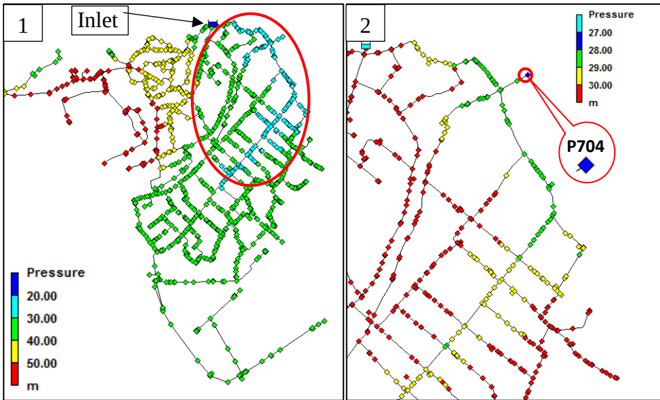
Figure 4.40. The location of the CP related to the least predicted pressure in the PSA (assuming +25% increase of non-leakage flow) during winter season. CP (P704), on 18.01.2016 at 01:50 PM; min. pressure = 27.81 m, \Sigma Q_{(125\% \times \text{non-leakage}) + (\text{leakage})} = 117.82 \text{ m}^3/\text{h} and pressure upstream PRV = 32.65 m
