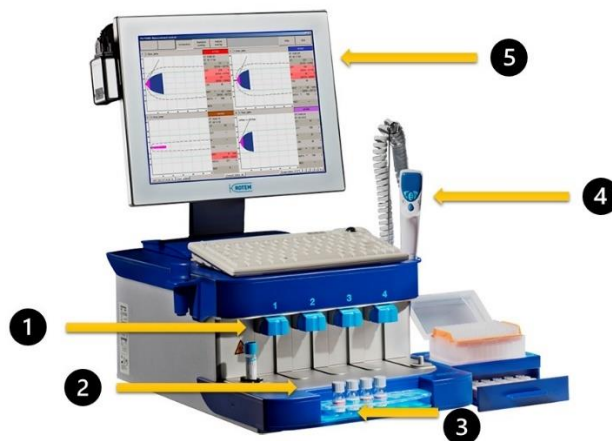
Figure 1. 6: ROTEM® delta device. This device consists of 1) a four-measurement unit with independent temperature-adjusted channels, 2) a pre-warming plate, 3) a reagent holder, 4) an automatic pipette, and 5) an integrated touch-screen computer.
