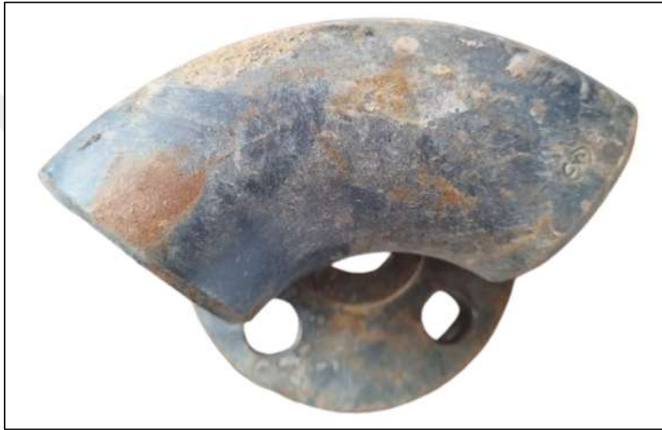
Figure 4.5: Visibly Detectable Rust Crack in an oil Pipe Section.
