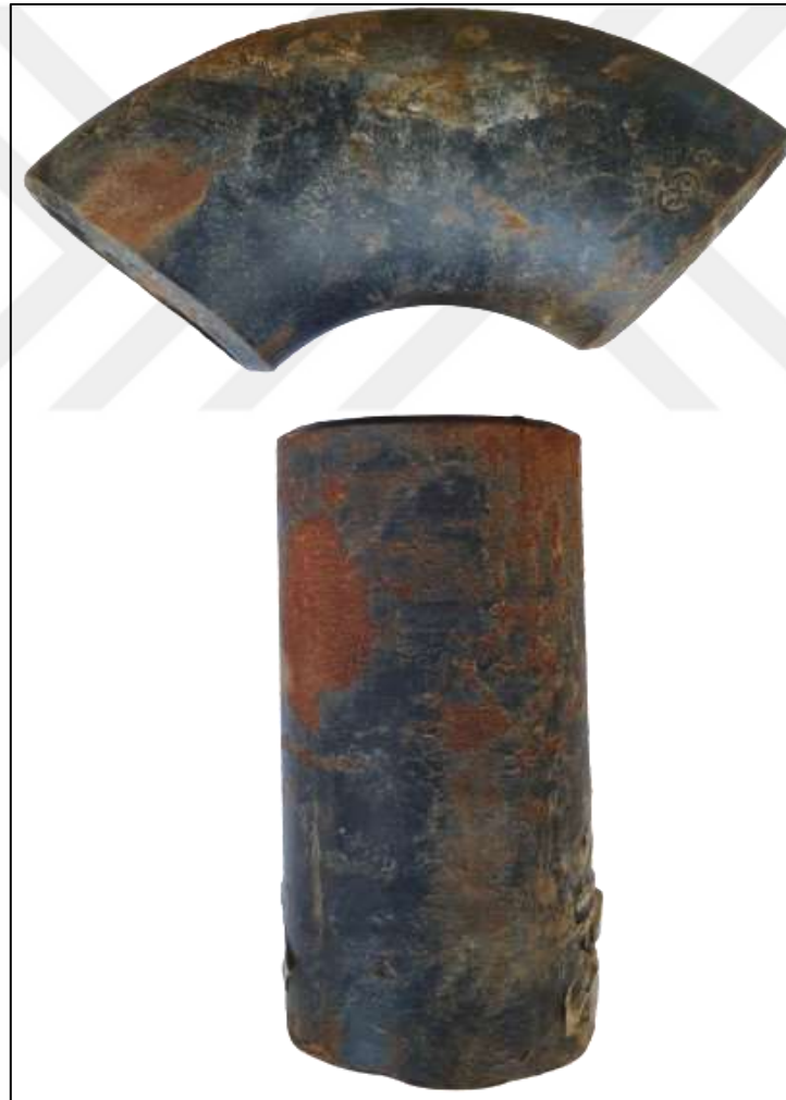
Figure 4.4: Rust Crack in a Pipe Section and Pipe Joint Taken from Beiji Refinery in Salahddin, Iraq.
