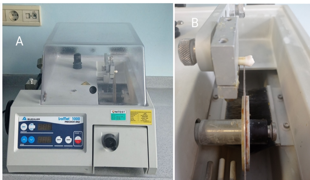
Figure 17: A. The diamond coated precision saw (Micromet 5114; Buchler, IL, USA) / B the tooth fixed in the machine 2 mm below the CEJ before sectioning.
