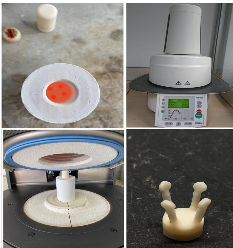
Figure 29: Pressing procedure for GC li si press ingots.
