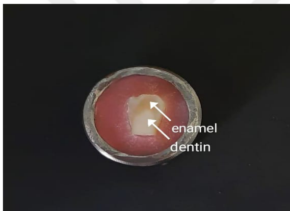
Figure 24: Preparation of enamel- dentin complex surface.
