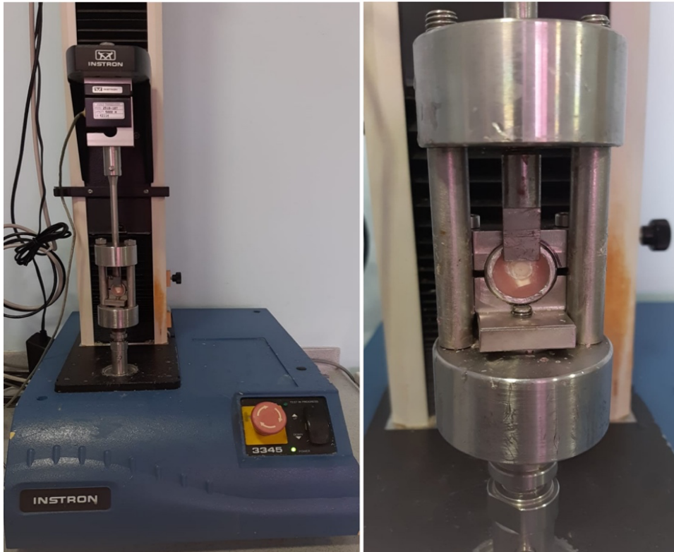
Figure 38: The samples fixed in the universal testing machine.
