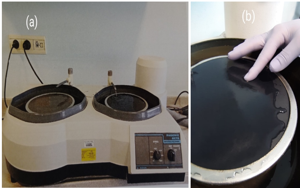
Figure 31: (a) Phoenix Beta Grinder \Polisher, Buehler, Germany.\ (b) Polishing of the porcelain discs.
