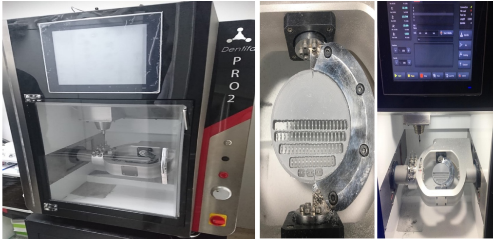
Figure 27: wax preparation of the porcelain in CAD-CAM machine.
