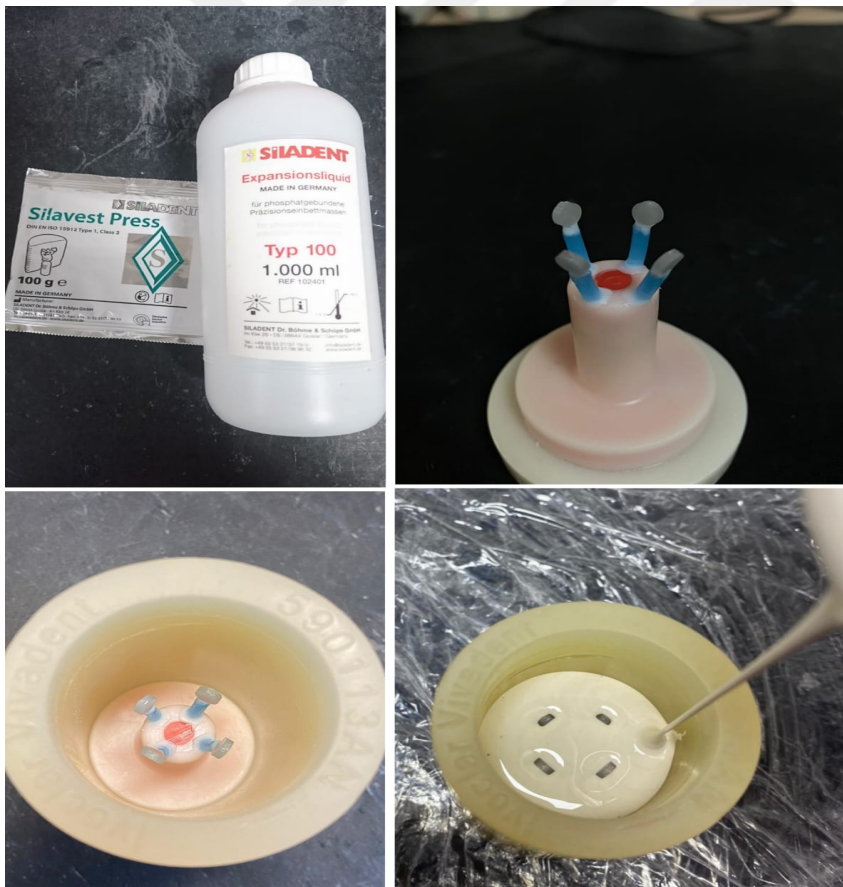
Figure 28: Investment procedure for the wax specimens.
