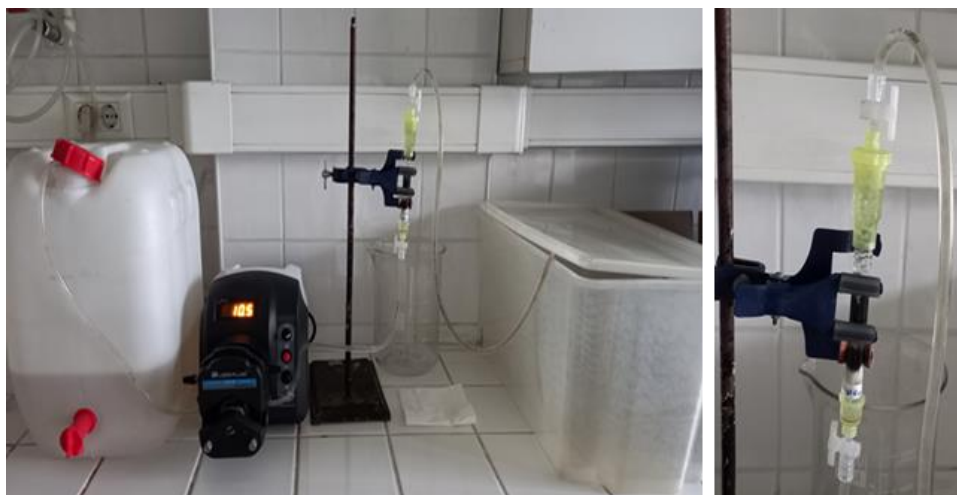
Figure 4.11. RSSCT set-up (left) and the small-scale GAC column (right).
