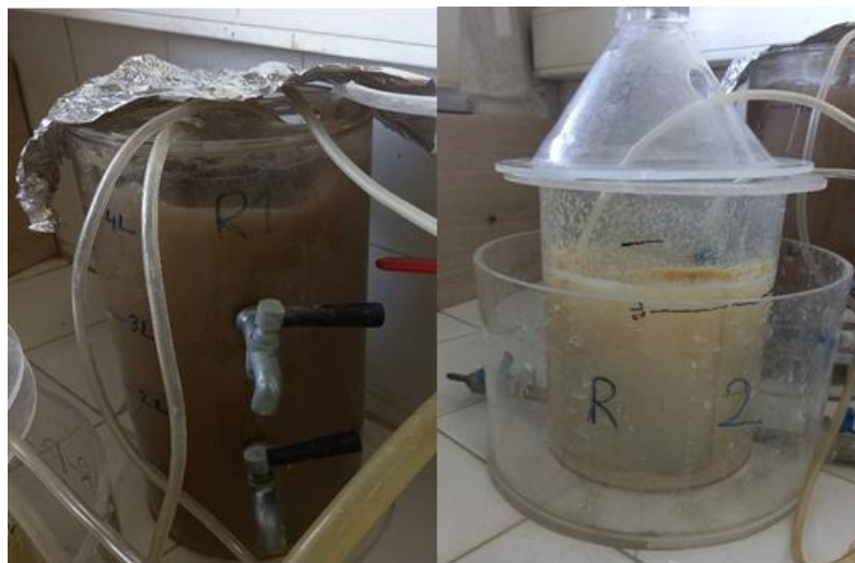
Figure 4.1. Activated sludge reactors (R1 and R2).
