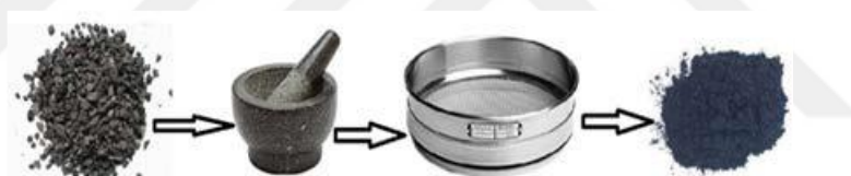
Figure 3.9. Schematic view of GAC grinding with a mortar and pestle.
