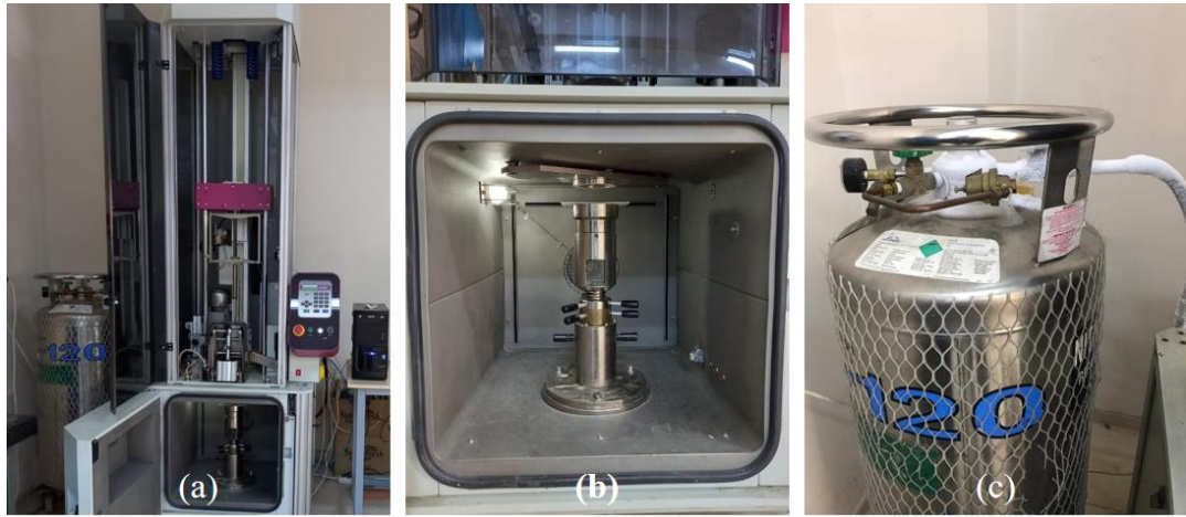
Figure 3.4 a) CEAST Fractovis Plus impact test machine, b) test specimen, c) liquid nitrogen tank (Personal archive, 2020)
