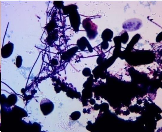
Microphoto 26: View of activated sludge Gram staining sample (third week), flocs, bundle of Gram positive filamentous bacteria, and eukaryotic cells, bright field microscopy, 1000X.
