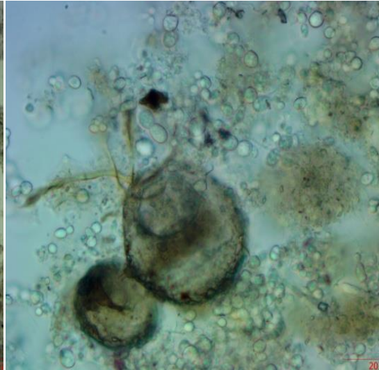
Microphoto 10: General view of activated sludge, flocs, eukaryotic cells, original wet mount sample (third week), bright field microscopy, 400X.
