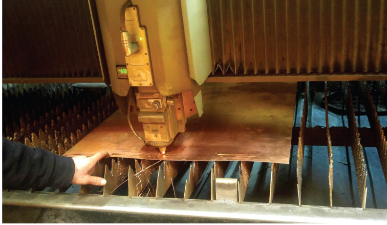
Figure 2.4: Manufacturing of flat wire from thin copper sheet using laser cutter
