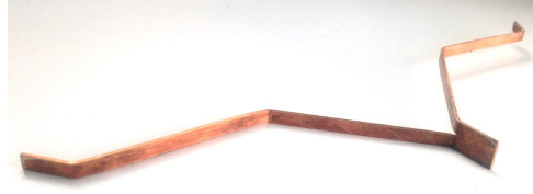
(b) Proposed flat wire made of thin conductor sheet
