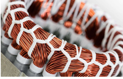
(a) Conventional winding with stranded round wires [2]
