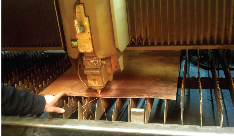
Figure 4.7: Manufacturing of flat wires with laser cutter
