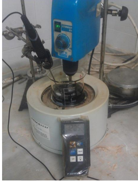
Figure 6.8 Production of WMA added bitumen using a heater (Personal archive, 2022)
