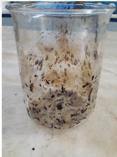
Figure 6.29 Glass beaker after bitumen draindown test (personal archive, 2022)
