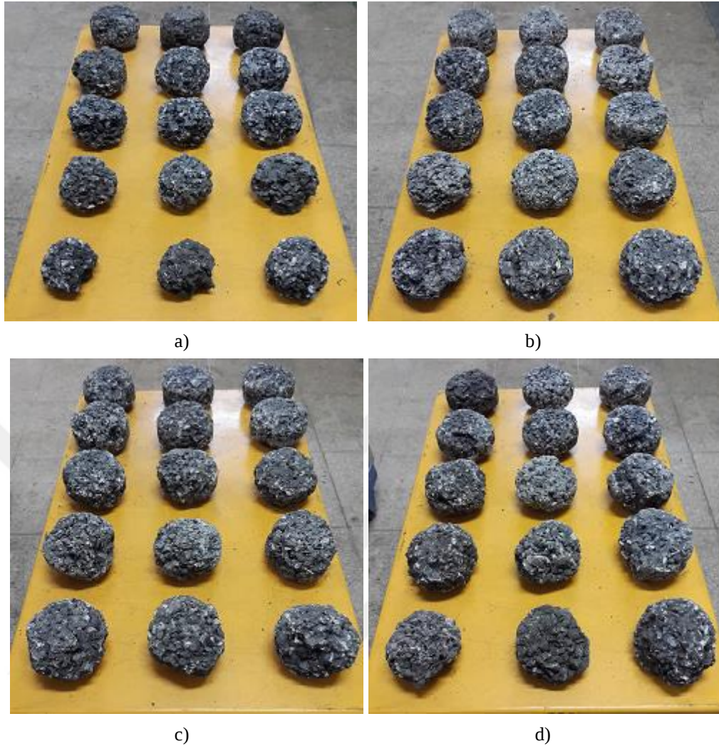
Figure 7.8 Samples after particle loss test prepared with limestone aggregate a) base bitumen, b) SBS pmb modified, c) Elvaloy pmb modified, d) Sasobit wma modified
