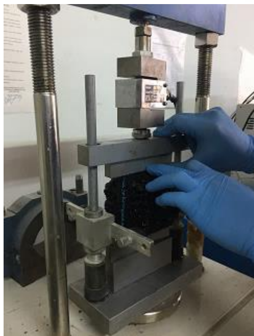
Figure 6.18 Loading the sample across the diameter (personal archive, 2022)
