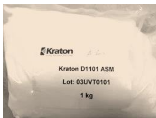
Figure 6.1 SBS Kraton® D-1101 (Powder Form) (Personal archive, 2022)
