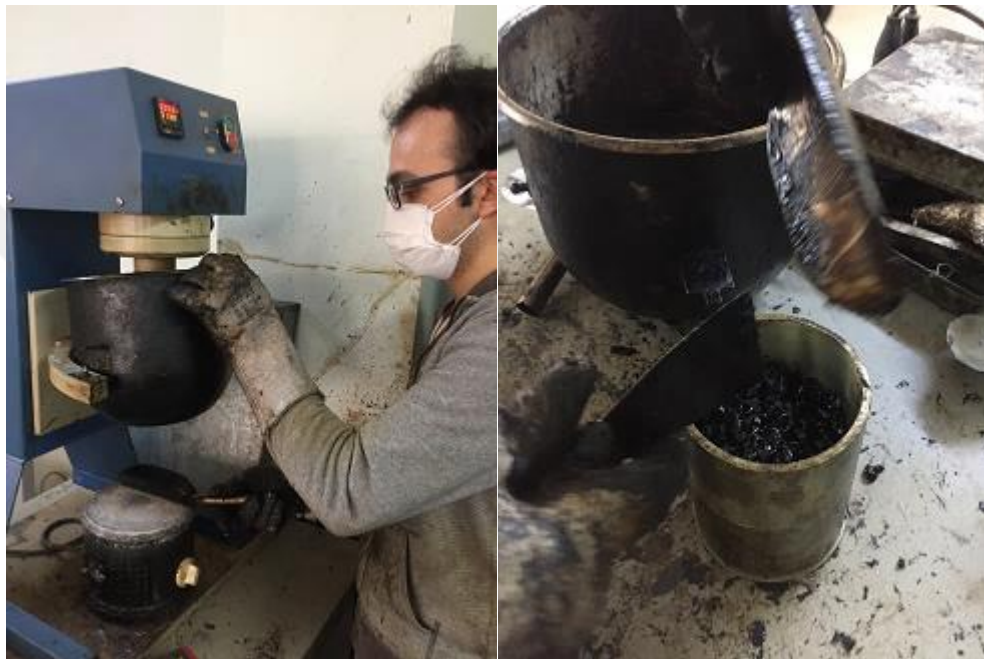
Figure 6.9 Mixing and placing materials (personal archive, 2022)
