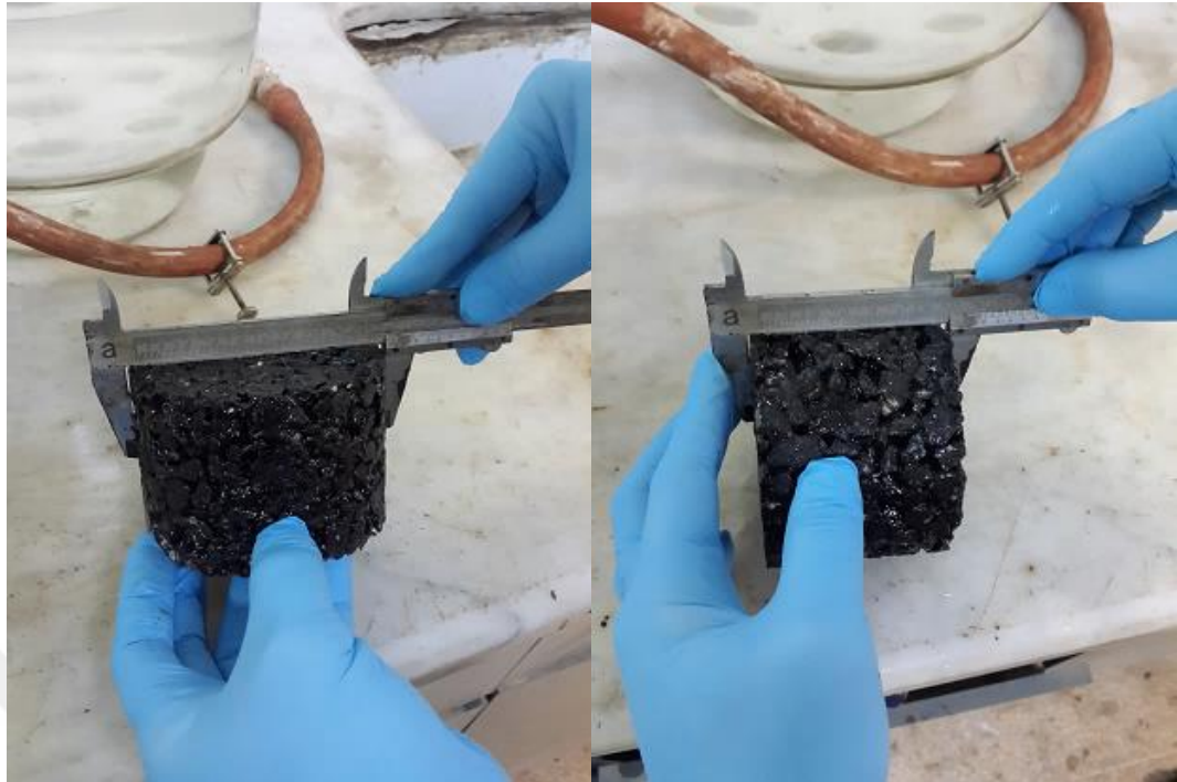
Figure 6.20 Measure the dimensions of the specimens (personal archive, 2022)
