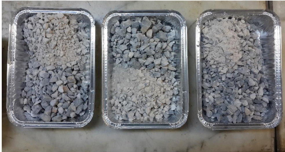
Figure 6.4 Aggregate weighing samples with limestone (Personal archive, 2022)
