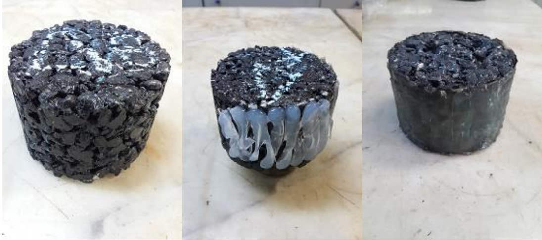
Figure 6.24 Covering the lateral surface with silicone (personal archive, 2022)
