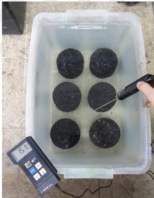
Figure 6.22 Water bath 4 hours at test temperature (personal archive, 2022)
