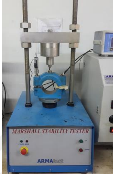
Figure 6.11 Marshall machine (Personal archive, 2022)
