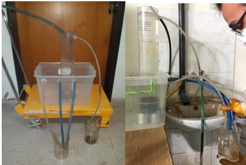
Figure 6.23 Permeability test arrangement (personal archive, 2022)
