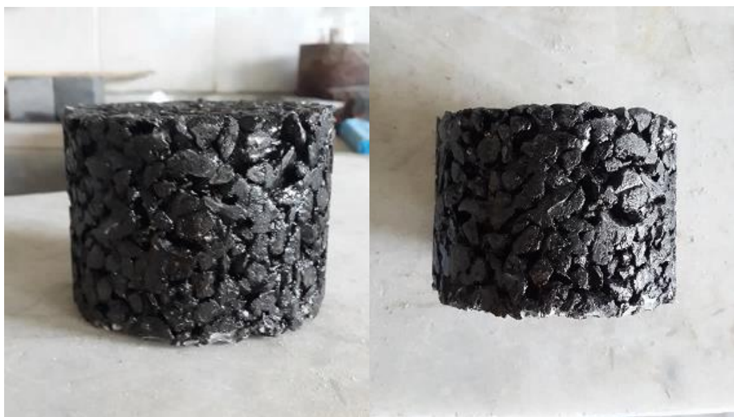
Figure 6.13 Sample prepared for particle (Cantabro) loss test
