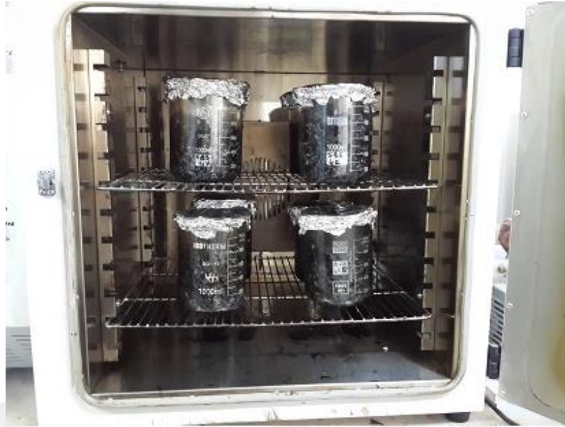
Figure 6.28 Keeping the mixture in an oven at 170 °C for 1 hour (personal archive, 2022)
