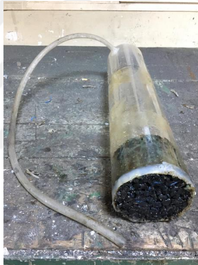
Figure 6.25 Fixing the sample to the water column for vertical permeability (personal archive, 2022)
