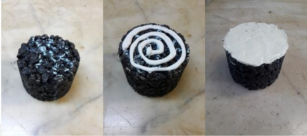
Figure 6.26 Covering the lower surface of the sample with silicone (personal archive, 2022)
