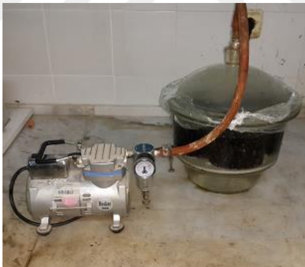
Figure 6.19 Apply a vacuum (personal archive, 2022)
