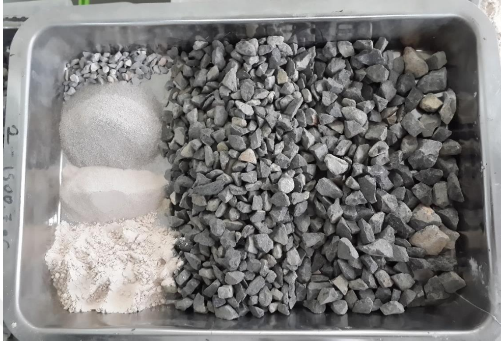
Figure 6.5 Aggregate weighing samples with basalt-limestone aggregate combination (Personal archive, 2022)
