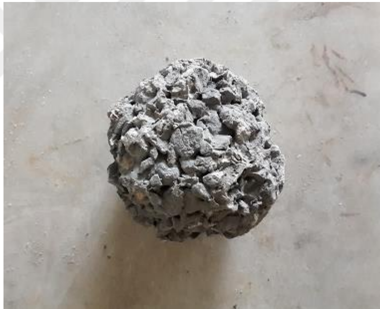
Figure 6.14 Sample after particle (Cantabro) loss test
