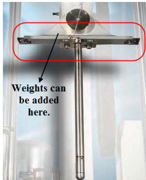
Figure 5.4 Weight adding unit.
