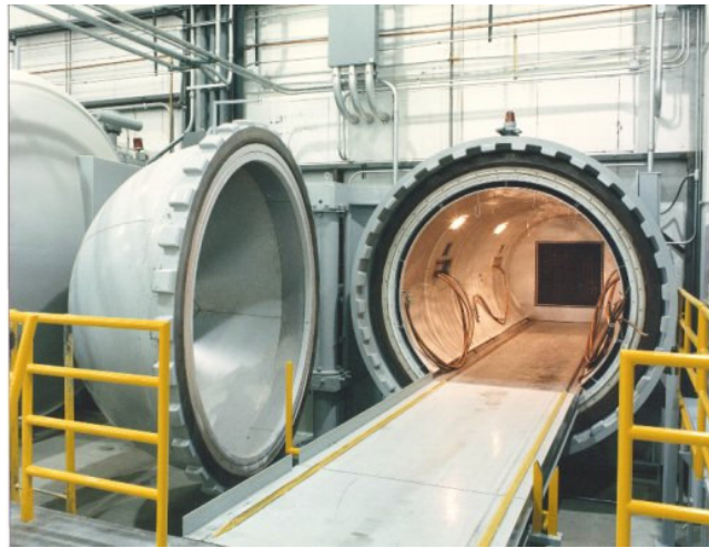
Figure 2.19 Autoclave for curing composites. ( www.aschome.com , 2008)
